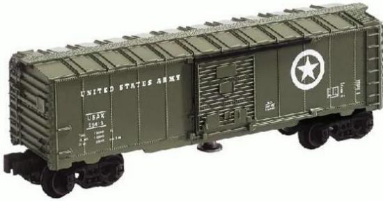
This is a modern era operational U S Army mail delivery box car. Using the uncoupling track, opens the door and the mailman “throws” out a mail sack. The car has a plastic body, sheet metal chassis, end brake wheel, and die cast sprung trucks with magnetic disk / tab couplers. Last catalogued in 2000. The Lionel catalog number is 6-26776
