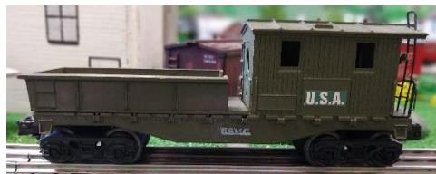
Modern era USMC work caboose with rear guard rail and ladder. Plastic body, chassis, and trucks. Couplers on both ends, no smoke stack.
