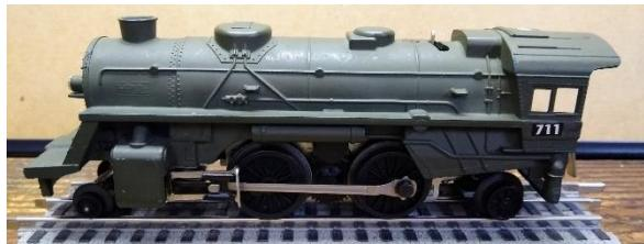
This Lionel locomotive is one of the items that were repainted in Olive drab for an army set. It is a repainted Lionel 8141 from the Pennsylvania Flyer Set. It would have been made in 1971 - 1972. This would be a very early Modern-MPC production. This plastic shell mold has been used by Lionel since the 1950s.
