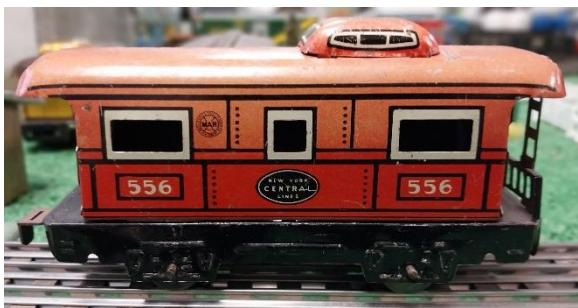
New York Central Red short SP style caboose, chassis mounted axles, rear guard railing with ladder, and slot / tab coupler.
