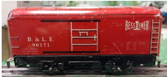
Pennsylvania Rail Road red short box car, chassis mounted axles, and slot / tab coupler. B. & L.E. is the Bessemer and Lake Erie Railroad that operated in northwestern Pennsylvania and northeast Ohio.
