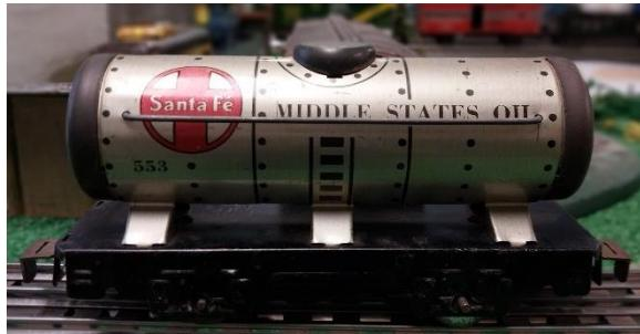
Santa Fe, Middle States Oil Silver short tank car, chassis mounted axles, hand rail, and slot / tab coupler
