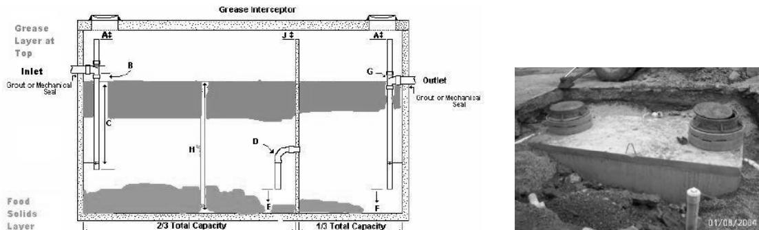
**Grease Trap** (under the sink & floor units)- make sure flow restrictor installed and properly vented.
